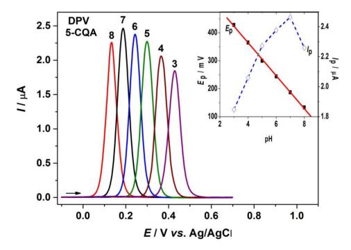
**Figure 4.** DPVs of  $5 \cdot 10^{-5}$  mol L<sup>-1</sup> solution of 5-CQA in 0.1 mol L<sup>-1</sup>PBS of different pH. Inset: Plots of  $E_p$  and  $I_p$  vs. pH. The experimental conditions for DPV are as in Figure 1.
