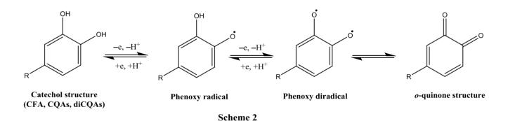
Scheme 2. Proposed mechanism for the electrochemical oxidation/reduction of CQAs, diCQAs and CFA
