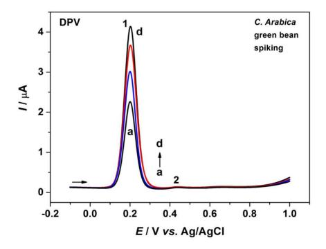
**Figure 6.** DPVs of *C. Arabica* green bean extract (diluted 50-fold), in 0.1 mol L<sup>-1</sup> PBS pH 7 (a). Spiked samples: (b) *C. Arabica* +  $3 \cdot 10^{-5}$  mol L<sup>-1</sup> of 5-CQA, (c) *C. Arabica* +  $1 \cdot 10^{-5}$  mol L<sup>-1</sup> of 3,4-diCQA, and (d) *C. Arabica* +  $1 \cdot 10^{-5}$  mol L<sup>-1</sup> of 4,5-diCQA. The experimental conditions for DPV are as in Figure 1.
