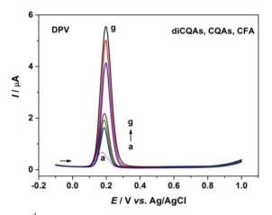
**Figure 1.** DPVs of  $3 \cdot 10^{-5}$  mol L<sup>-1</sup> solution of: CFA (a), 5-CQA (b), 3-CQA (c), 4-CQA (d), 3,4-diCQA (e), 3,5-diCQA (f), and 4,5-diCQA (g), in 0.1 mol L<sup>-1</sup> PBS pH 7. The experimental conditions for DPV measurements were: pulse amplitude 50 mV, pulse width 70 ms, potential increment 2 mV, interval time 0.4 s, scan rate 5 mV s<sup>-1</sup>.
