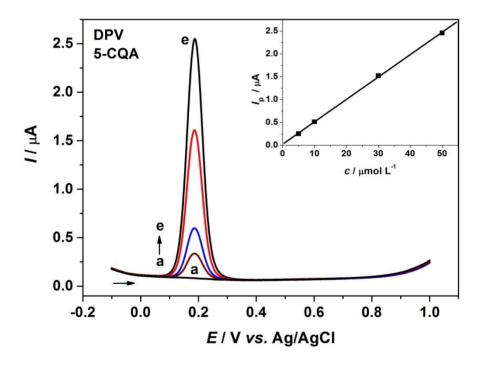
**Figure 5.** DPVs of 5-CQA solutions of different concentration: 0 (a),  $5 \cdot 10^{-6}$  (b),  $1 \cdot 10^{-5}$  (c),  $3 \cdot 10^{-5}$  (d), and  $5 \cdot 10^{-5}$  mol L<sup>-1</sup> (e), in PBS of pH 7. Inset: calibration plot of 5-CQA. The experimental conditions for DPV are as in Figure 1
