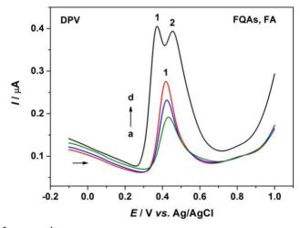
**Figure 2.** DPVs of  $3 \cdot 10^{-5}$  mol L<sup>-1</sup> solution of: 4-FQA(a), 3-FQA (b), 5-FQA (c), FA (d) in 0.1 mol L<sup>-1</sup> PBS pH 7. The experimental conditions for DPV are as in Figure 1.
