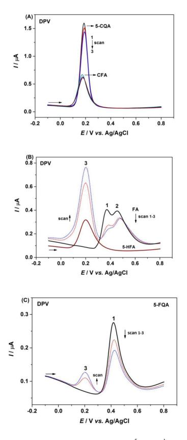
**Figure 3.** The effect of successive scans on DPVs in 3·10<sup>-5</sup> mol L<sup>-1</sup> solution of: 5-CQA and CFA (Figure 3A), FA (Figure 3B), and 5-FQA (Figure 3C) in 0.1 mol L<sup>-1</sup> PBS pH 7. The experimental conditions for DPV are as in Figure 1.
